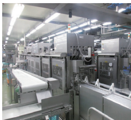
"YIELDAS," a fully automated chicken deboning machine
